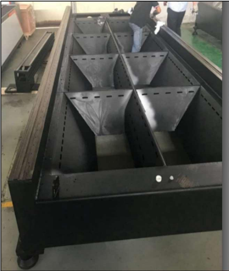
➤ LASER CUTTING MACHINE BED
